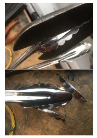
Cut each side off the existing round end straight toward the heel removing all the scallops.
