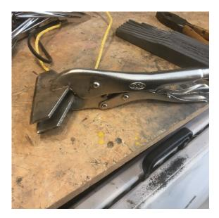
Set it to clamp about 13mm and re-bend each blade to form a half tube.
