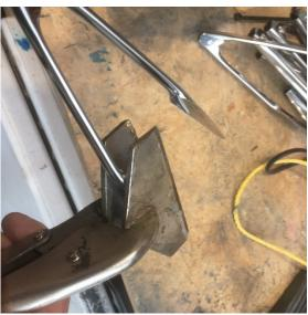
Squeeze and rotate the ends so they form a symmetrical half circular tip.
