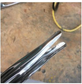
Put a 15mm spacer between the handles and rebend the ends of the blades so they touch. I used the handles of the pliers.
