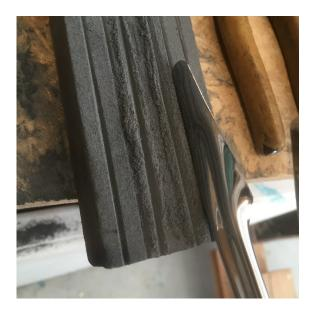
100mm welding edge clamp from Supercheap Auto.
