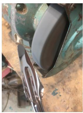
Use fine wheel and lightly grind off to remove the cut bur.
