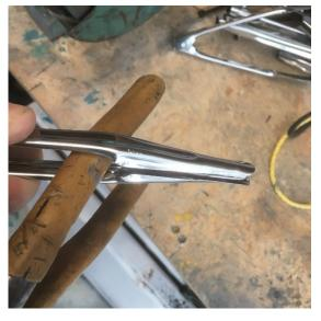
Now when the dibblers are closed they meet to form the metal cone required to protect the tap root and prevent damage and J-root. About 0.75cm when closed seems to work well, but a larger one also works on grasses, iris where more than one plant is good.
