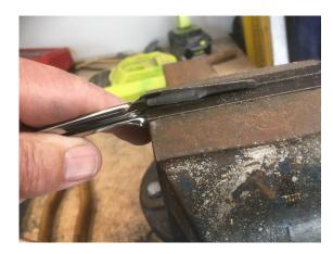
The vice allows pressure to be put on the stainless steel. Repeat for all four edges.
